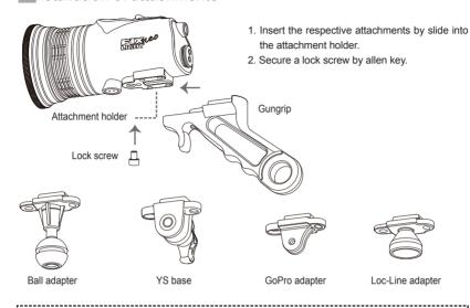
**NOTE** Using wrist lanyard is recommended to prevent of loss.
